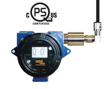
The GDS-58X explosion-proof wireless 4-20mA State Transmitter accepts normally-open or normally-closed switch contacts and broadcasts them on GDS Corp wireless networks.
