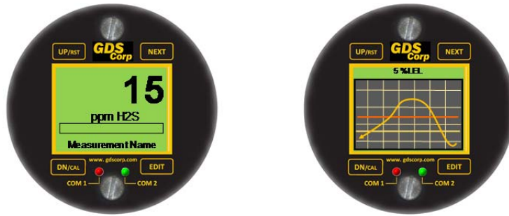
Figure 5-1: GDS-78XP GASMAX Display Sequence: Display Screen & Trend Screen
