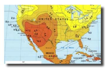
Note: Solar power output varies with geographic location and time of year. Power specifications are based on proper installation in winter sun in locations defined as "4.5" shown above. Actual power output may be higher or lower then specified. Contact GDS Corp for an analysis of your solar power requirements or for a fully custom system designed to meet your exact needs.
