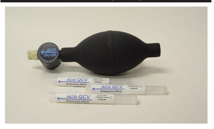
The QC-50 from Advanced Calibration Designs provides a quick and easy method of checking the performance of gas detection systems. The QC-50 utilizes revolutionary technology allowing a functional check (or 'Bump Test') as needed or required by law. The unique QuickCheck Vials (QCV) utilize a stable, safe and reliable delivery method allowing ease of shipment, storage and use. The QC-50 is currently available for ammonia, hexane, hydrogen chloride and toluene.
