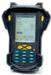
Hand Held Diagnostic Unit p/n 12-0450 Certified I.S. (EExia) for use in hazardous areas.
