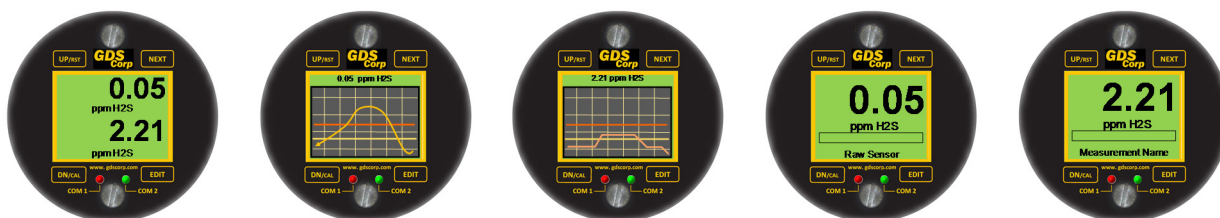
Figure 6-4: GDS-68XP GASMAX Display Sequence
